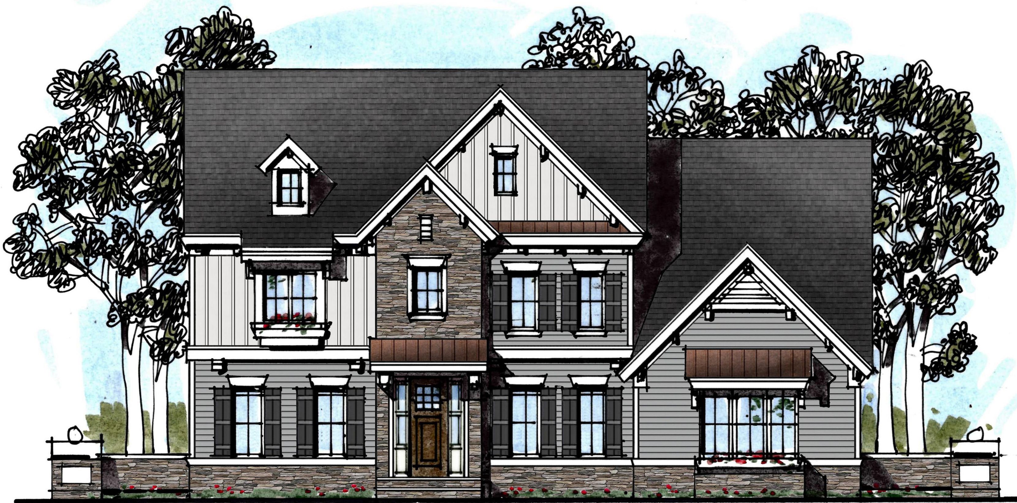
FRONT ELEVATION STONE | SIDING | VERTICAL SIDING
